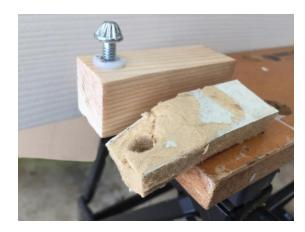
Hole in bottom of opposite panel was used to transfer location of leveler hole to our block of wood.
